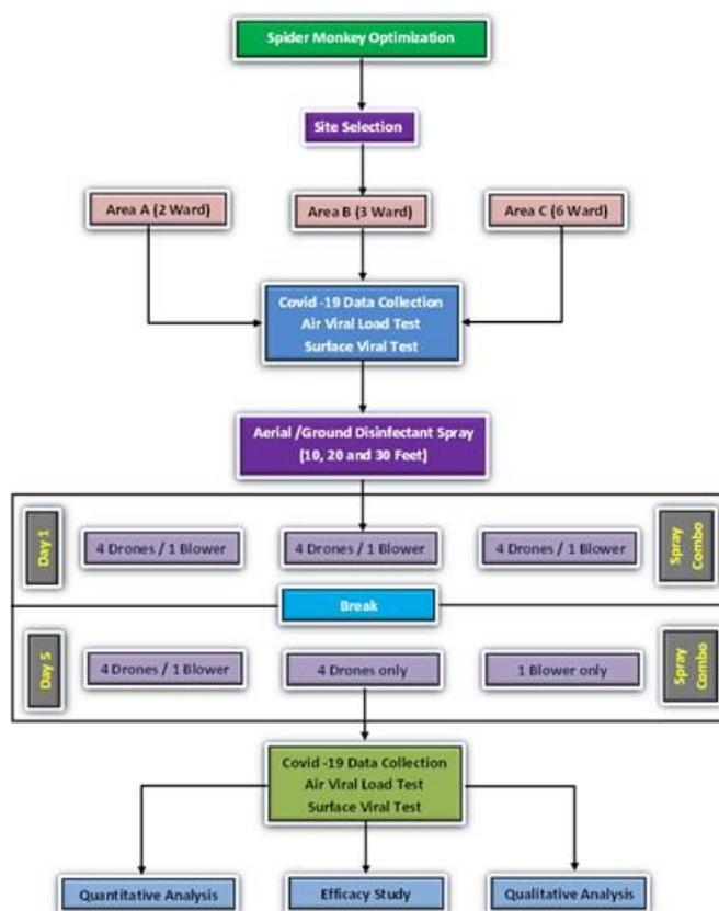
Fig. 4. Adopted Methodology for Sugaradhana Organic Disinfectant Spray using Drone and Mist Blower
