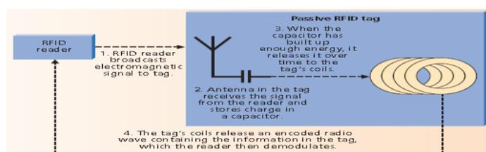
**Fig5.2. Working of RFID**
